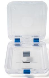
**PN** PR001820 | Step height 1 µm (Sensofar traceable)
