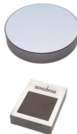
Calibration specimen designed to calibrate Ai Focus Variation and Confocal Continuous techniques. The nominal roughness is  $S_a$  0.80  $\mu\text{m}$ . The engraved area size is 20x20 mm.
