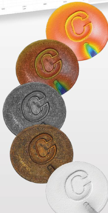
Five smart visualization modes (false color, stack, stack & false color, true color or directional luminance) are always within reach in the main screen.
