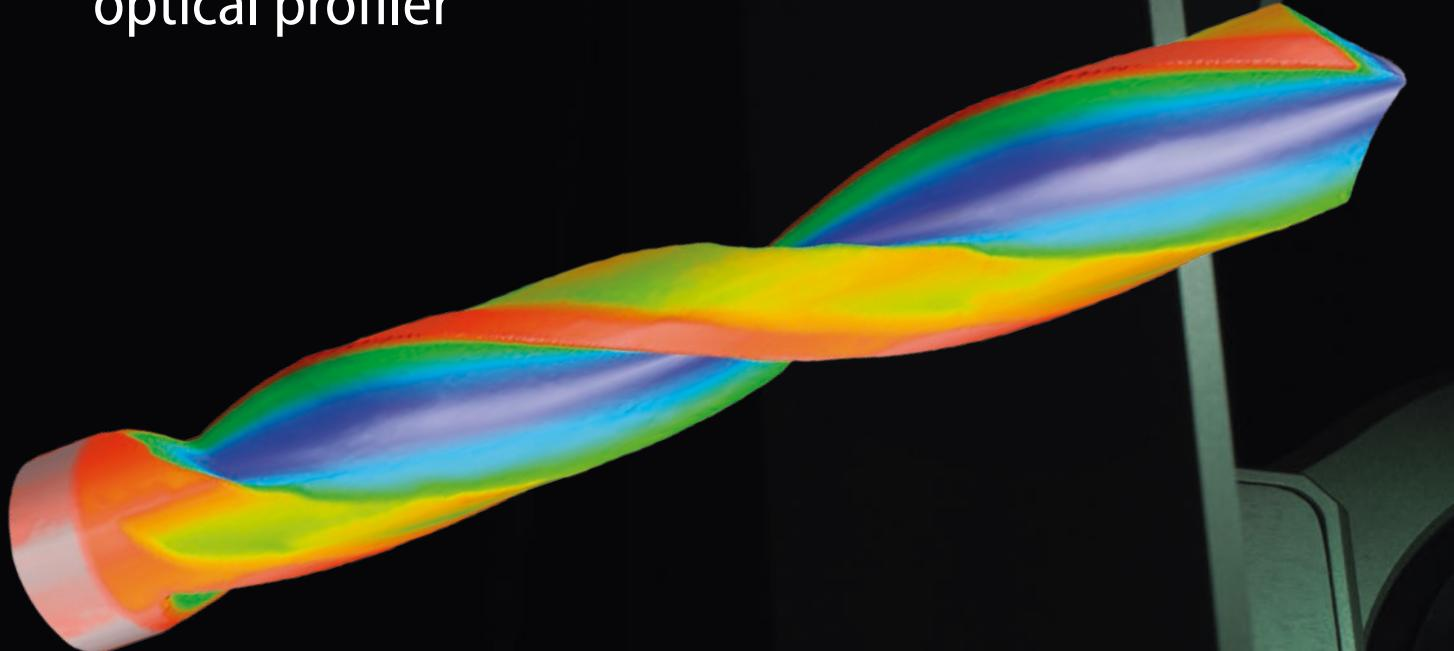
This enables automatic 3D surface measurements at defined positions which can be combined to create a complete 3D volumetric measurement. S neox 3D measurement technologies cover a wide range of scales, including form (Ai Focus Variation), sub nanometric roughness (Interferometry) or critical dimensions that require high lateral resolution as well as vertical resolution (Confocal).
